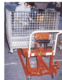
Improve efficiency by lifting mesh pallets to remove items underneath them
